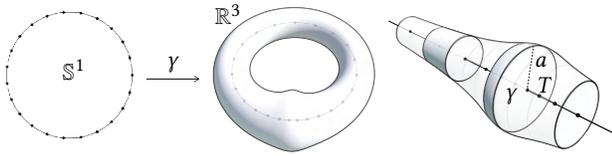
Fig. 6. Geometry of a variable thickness vortex filament described by its center curve  $\gamma$  together with a radius function  $a > 0$ . The full vortex filament is then the embedded solid torus swept out by disks of radius  $a$  normal to the tangent  $T$  along  $\gamma$ .
